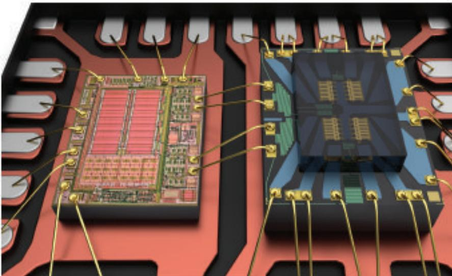
Figure 5. Drive IC (left), MEMS switch die (right) mounted on and wire-bonded to a metal lead frame
