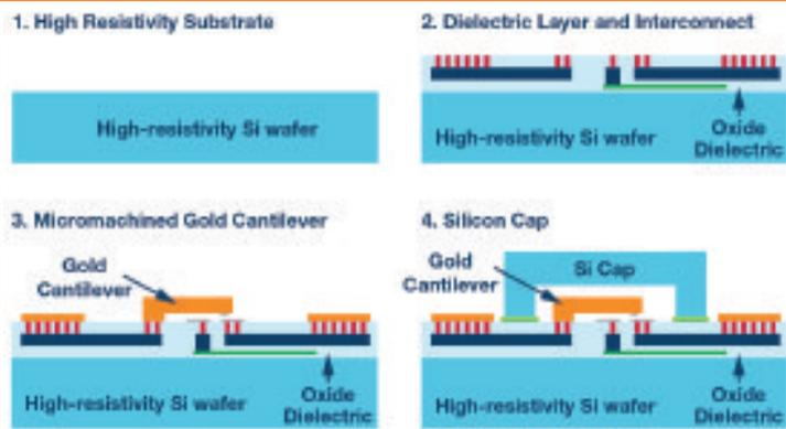
Figure 3. MEMS switch fabrication overview
